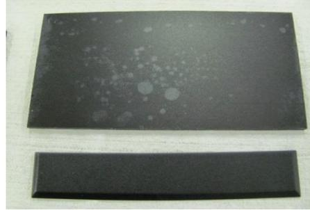
Coating 1 coated with insufficient UV energy
