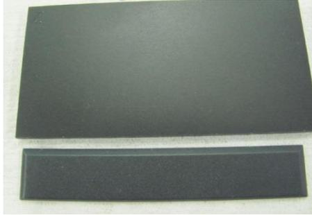
Coating 1 processed within thickness, flash off and UV energy recommended ranges
